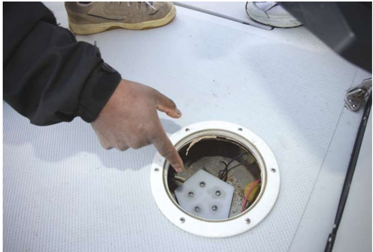
In addition to giving boat operators a highly accurate reading of fuel levels, this sensor detects water in the bottom of the tank, whether it is mixed with ethanol, gasoline, diesel, or two-stroke oil.
