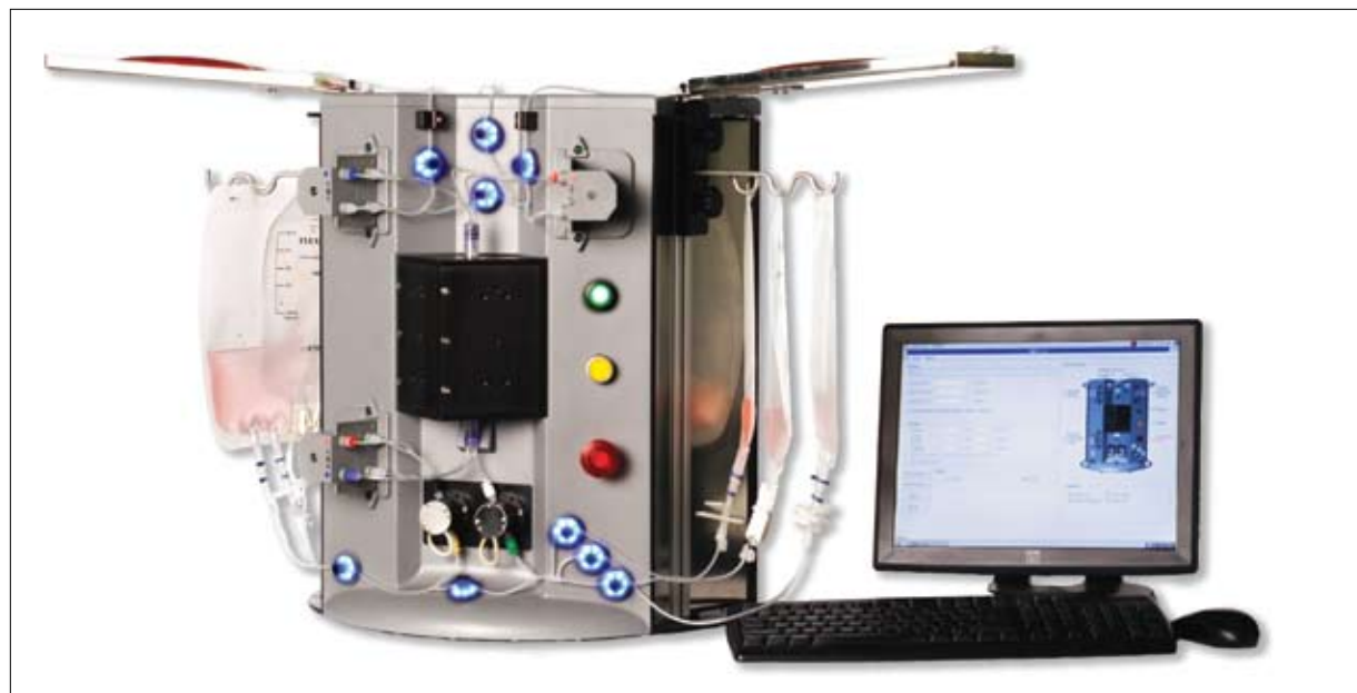
Techshot and IKOTech licensed and commercialized this Quadruple Magnetic Sorter, which uses magnetophoresis for cancer research and stem cell processes.
